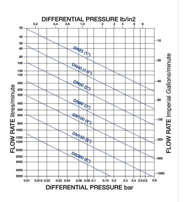
The chart is for water (1cSt) flowing through a filter with an element coarser than 1 millimetre perforations. Multiply the chart pressure drop by the following factors for different ratings and different viscosities to calculate the actual pressure drop.
